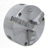
These chucks are available with 3 jaws, 4 jaws and 6 jaws and are referred as STC-3, STC-4 and STC-6 respectively. STC-3 chucks are most popular. STC-4 chucks are used when the job is square. STC-6 chucks are used to grip jobs having thin walls as holding pressure is divided on six sides. One set of reverse Jaws, Mounting Bolts, Operating Key and Inspection Report is provided with each chuck
